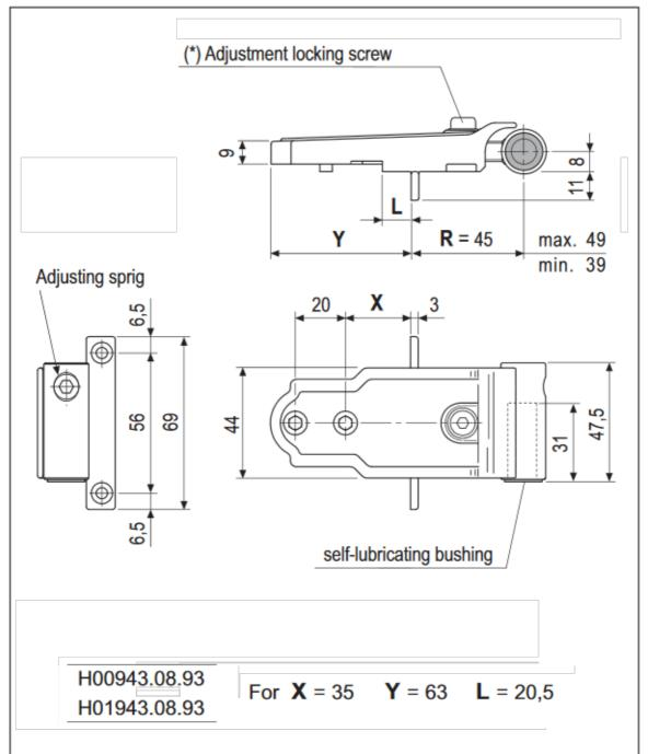
(\*) Before adjusting the hinge, make sure the screw is not locked.
